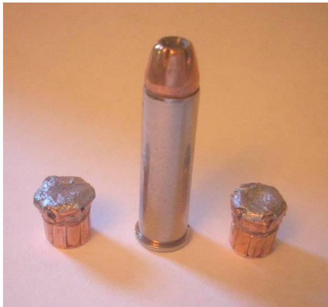
.357 Magnum shells (Left): from victim (Center): new, not fired (Right): test fire shell from Python in evidence locker
